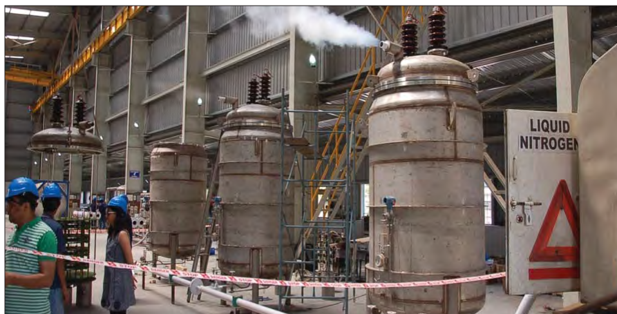
Trial for 3 Phase Superconducting Fault Current Limiter. Image: Shell -N-Tube
